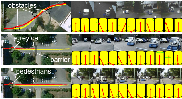
Fig. 3. Top to bottom: experiments 1 to 3. Left: reconstruction of the replayed path with (red) and without (yellow) obstacles. Right: snapshots (above) and grids (below) in the presence of obstacles. The red vectors show the orientation of f .
