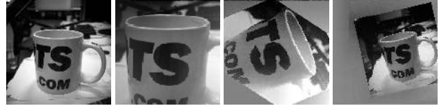
Figure 2: Examples of in-plane image transformations performed on SCAMP-5. L-R: original, zoom-in, zoom-in+CWrotate and zoom-out+CCWrotate+Rshift
