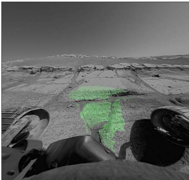
Figure 9. After Opportunity's 8.7-m slope drive on Sol 304, the goal area is perfectly reachable inside the IDD work volume, indicated in green.
