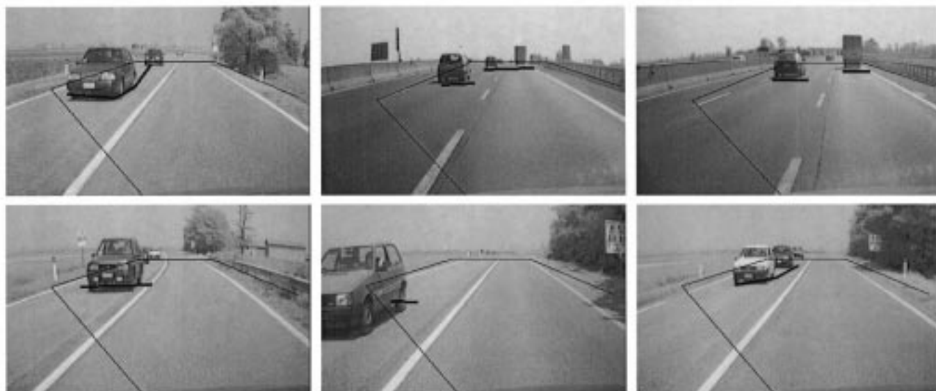
Fig. 3. Obstacle Detection. Result is shown with a black marking superimposed onto a brighter version of the image captured by the left camera; a black thin line limits the portion of the road seen by both cameras.
