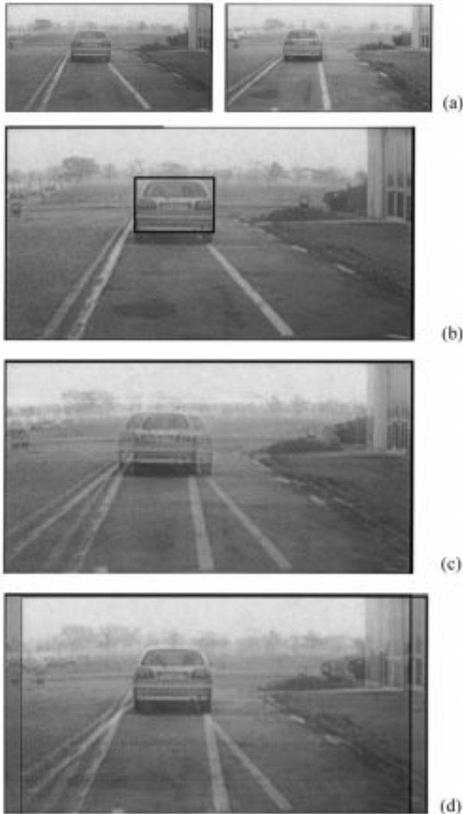
Fig. 17. Distance refinement: (a) left and right stereo images; (b) incorrect result of the detection step (the lower part of the bounding box indicates a wrong distance); (c) superimposition of stereo images with a null offset; and (d) superimposition of correctly shifted stereo images.
