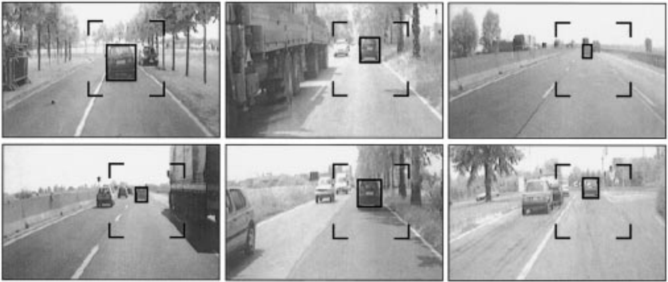
Fig. 18. Vehicle Detection: the images show the search area and the detected vehicle with black markings superimposed onto a brighter version of the original image.
