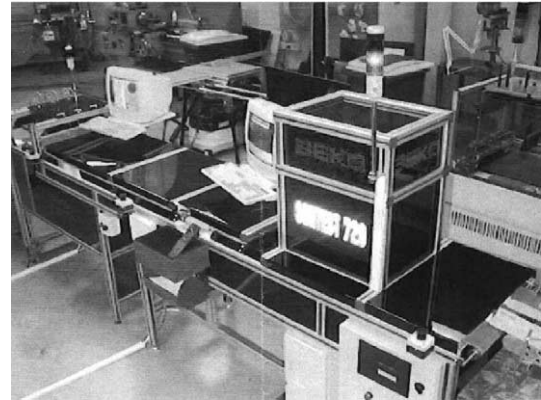
Fig. 13. Automated sorting system (courtesy of Beko A.Ş.). From the right part, remote controllers are fed automatically one-by-one from the assembly line. A camera acquires their image and visual processing determines their type. Accordingly, the remote controllers are directed to one of the control stations. Those whose types are unidentified are directed to a basket as seen in the front.
