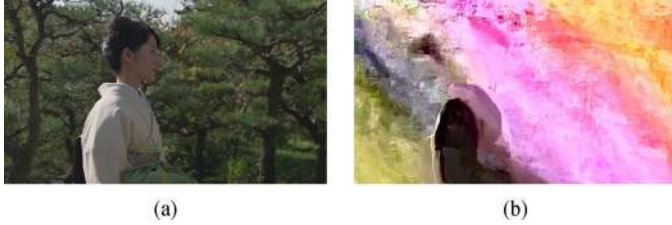
Fig. 8. Key sensitivity test for kimono #0. The SE frame is decrypted with: (a) Original key: PSNR (YUV) = {45.78, 47.04, 48.88} dB, (b) 1-bit different key: PSNR (YUV) = {9.45, 19.11, 13.63} dB.
