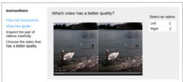
Fig. 3. Interface of crowdsourcing experiment. By clicking the play button, a pair of videos will be played simultaneously. Turkers (i.e., crowd workers working via AMT) were asked to identify and select the video with better quality for each video pair (forced binary choice). They can playback the pair of videos several times as they want.
