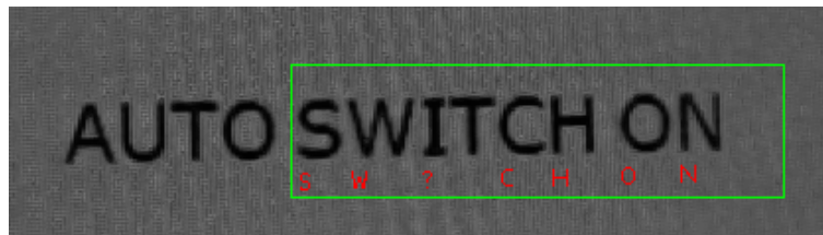
Figure 19. Original recognition result (missing letters: “T” and “T”).
