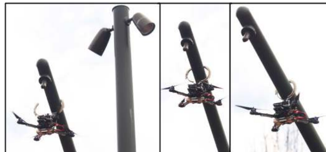
Fig. 1. A sample outdoor perch location for a quadrotor on a cantilevered cylindrical light post. Note that the axis of the cylinder can generally oriented.
