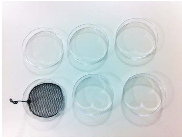
Figure 6.1 Petri dish set for change of solutions for the immunohistochemical protocol with the plastic mesh designed for handling the free floating retinal wholemounts.
