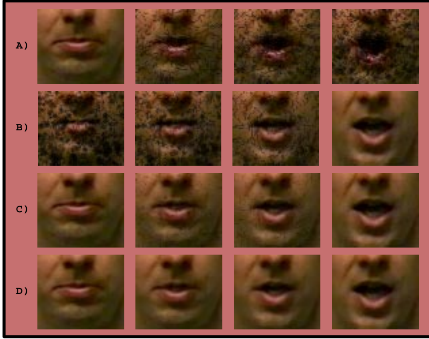
Figure 7. A) Forward warping viseme I_0 (first image) towards I_1 . B) Forward warping viseme I_1 (last image) towards I_0 . C) Morphing the images in I_0 and I_1 together. D) The same morphed images as in C), after hole-filling and median-filtering. Note that our morphing algorithm operates on the entire facial image, although we only show the region around the mouth for clarity.
