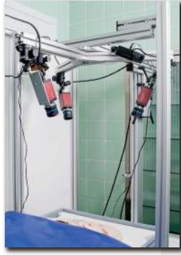
Fig. 3. Experimental setup for evaluation of the image stabilization performance. The motion of the pressure-regulated artificial heart is measured by a trinocular camera system.
