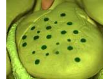
Fig. 4. The measured positions of the small green markers are used for evaluating the visual stabilization and therefore, they are not considered by filtering. The measured positions of the large green markers are included in the measurement vector \hat{\underline{f}}_k .
