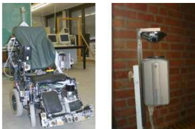
Figure 1: Left: the wheel chair test platform. Right: the omnidirectional camera system.
