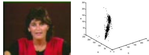
Figure 1. An example of a face image and the skin-color occurrences in the RGB space
