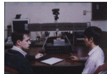
Figure 9. Setup of microphone array and face tracker
