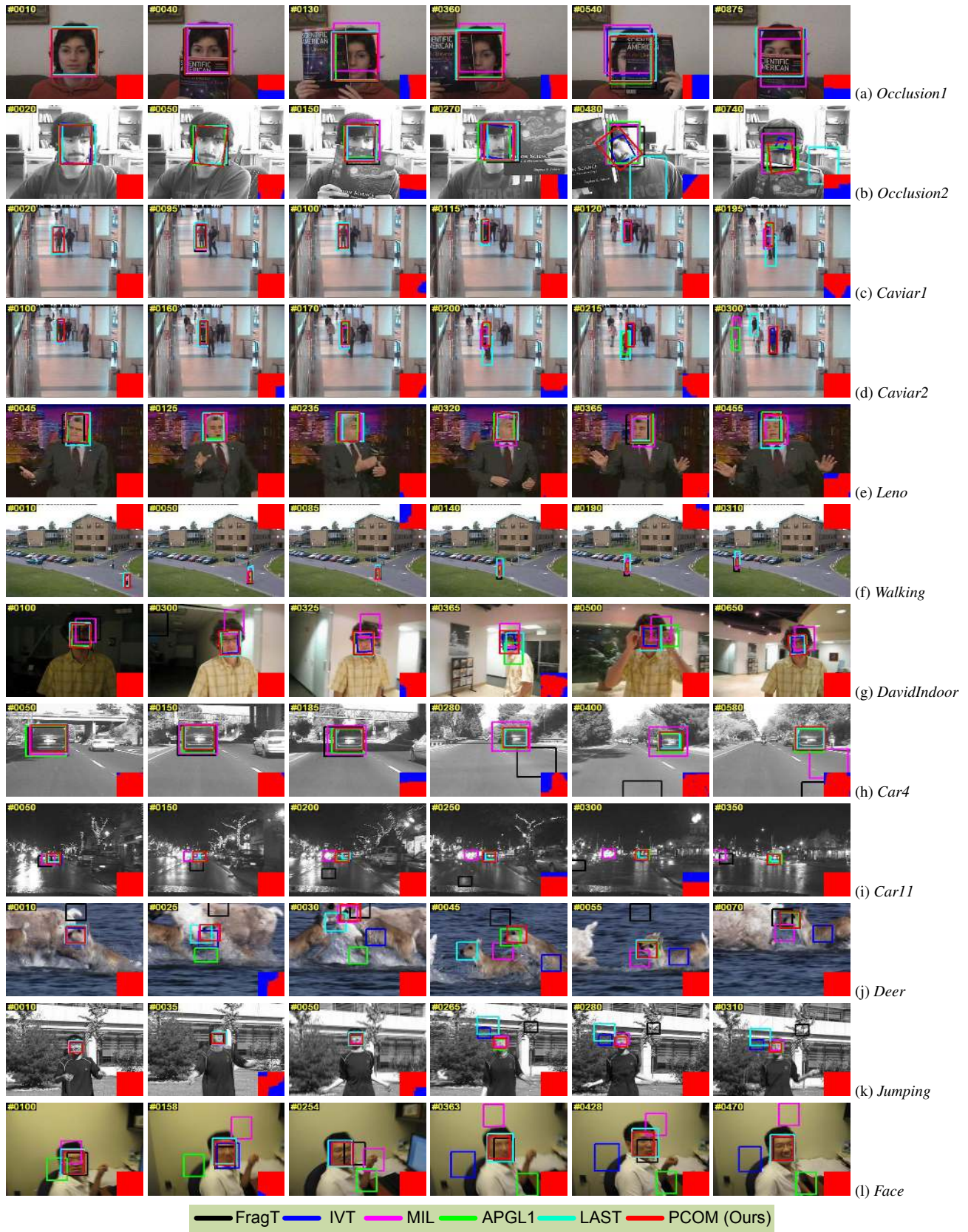
Figure 4. Qualitative evaluation of different tracking algorithms on twelve challenging image sequences. The estimated inlier-outlier masks are shown in the lower right (or upper right) of each frame, where the red color stands for inliers and the blue one indicates outliers.
