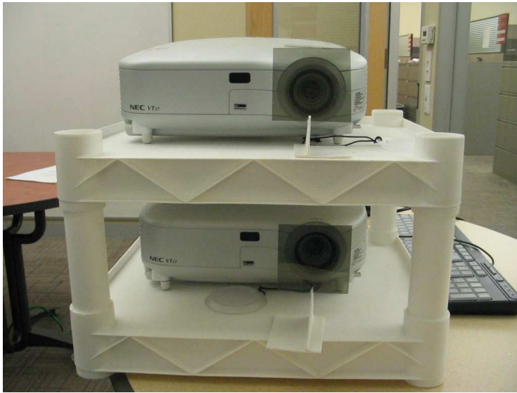
Fig. 13. The dual-channel polarized projectors for overlaying the simulated results on the observation data.
