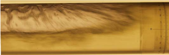
Figure 5. Photograph of slug tail (flow left to right).
