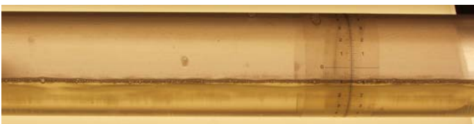
Figure 6. Stratified flow (flow left to right).
