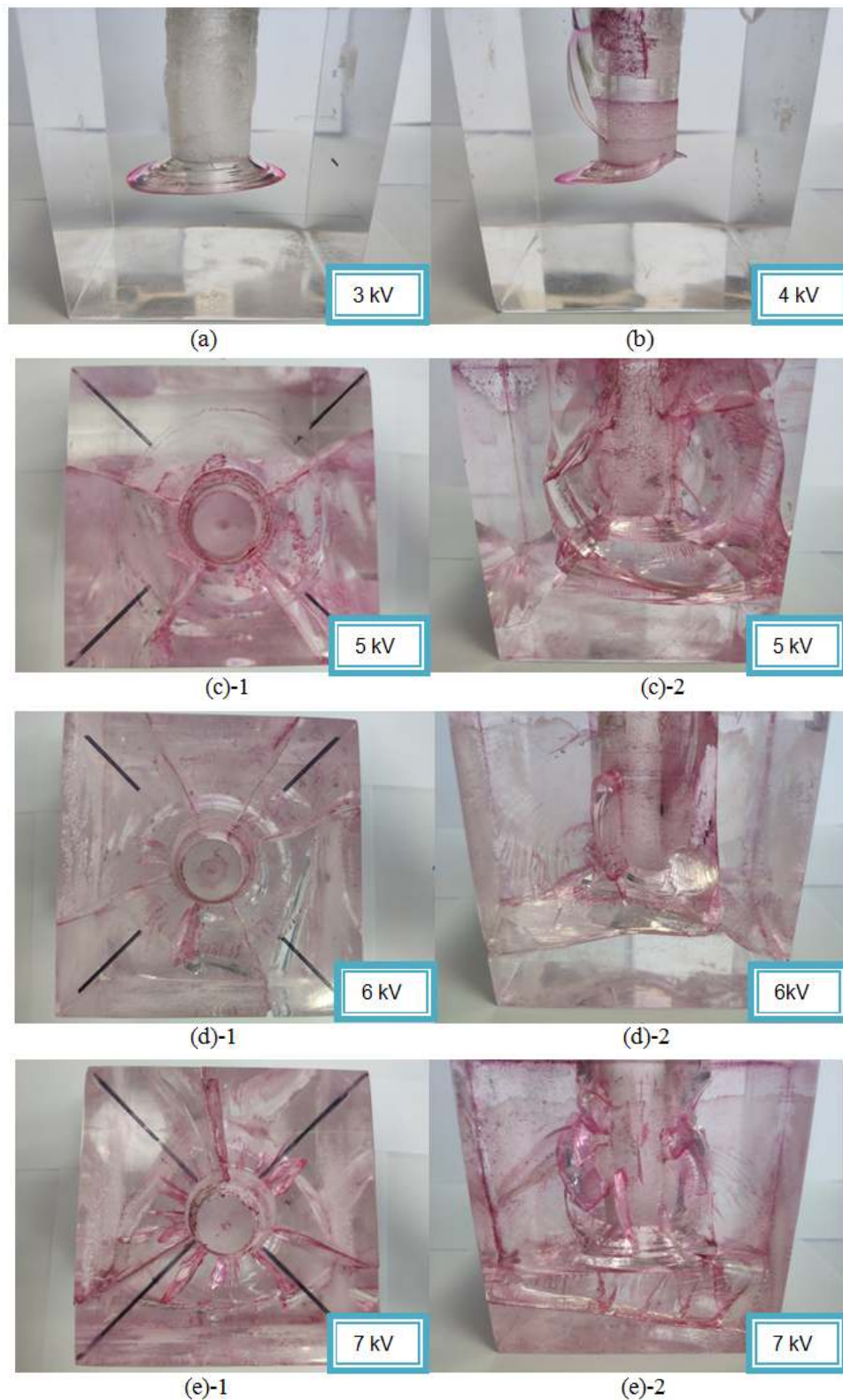
Fig. 4. Experimental PMMA fracturing results for each group
