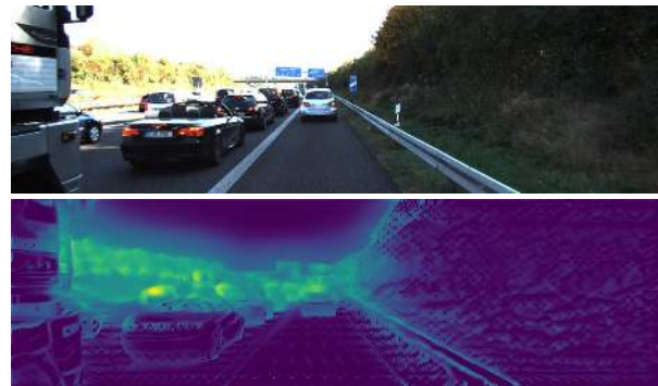
Figure 1. An example of the proposed visualization of single view depth estimation. Upper: an input image. Lower: a mask generated by our method showing relevant pixels for depth estimation.
