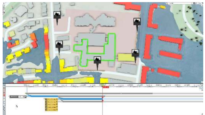
Fig. 8: A World Lines view (bottom) shows the history of a flood simulation (top) and allows the user to steer and compare the simulations. This greatly enhances the ease with which users can compare management strategies [18].
