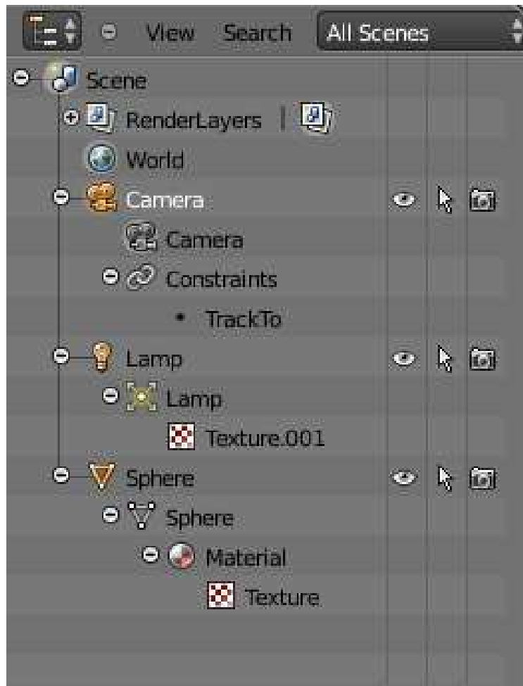
Fig. 10.— Data outliner widget. This hierarchical tree view depicts the program’s outline of all objects within the scene. In this example, the Camera has a "Track To" constraint applied. The map has a simple lighting texture, and the sphere (a planet in this case) has a material and UV-mapped texture applied. Each object is displayed in the view port, indicated by the eye icon. Each object is also applied to at least one render layer, indicated by the camera icon on the right hand side.
