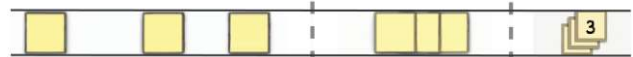
Figure 15. Screenshot of the prototype: During panning proxy elements (left) can overlap (center). If the user stops panning the overlapping proxies are animated towards each other and a cluster proxy appears (right).
