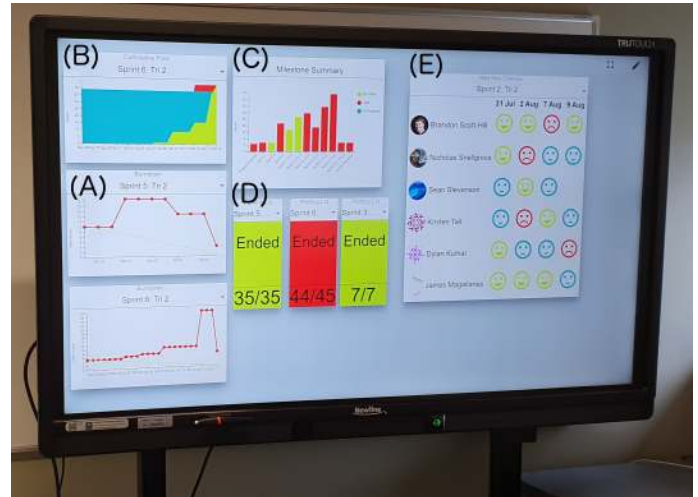
Fig. 1. DashVis on large touch display (65 inches) with visualizations: A) Burndown Charts, B) Cumulative Flow Diagram, C) Milestone Summary Chart, D) Parking Lot Diagram, and E) Niko Niko Calendar.
