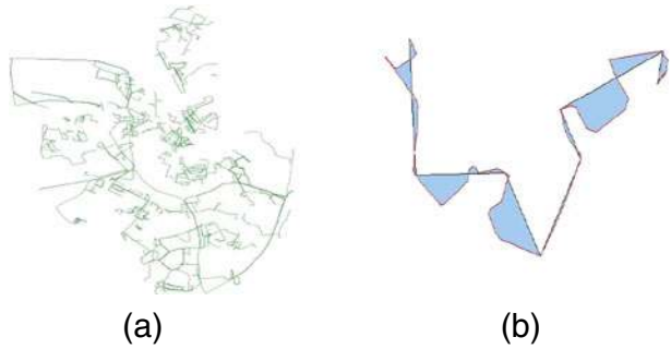
Fig. 18 a Synthetic dataset S_0 generated on Oldenburg's road network, b the route of a trajectory (black polyline) and its compressed counterpart (red polyline)
