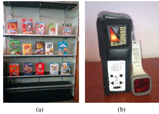
Figure 9: (a) Our mock grocery store shelf stocked with 15 different cereal boxes. (b) The ID Mate II talking barcode scanner from Envision America.
