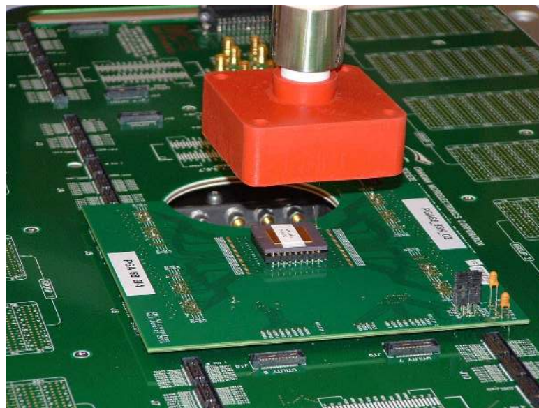
Figure 5.15: Test setup using Verigy 93K tester, Temptronic TP04300 thermal forcing unit head, and the DUT.
