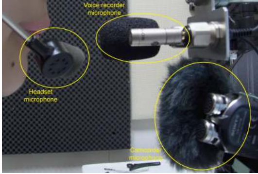
Figure 5: Six microphones are used simultaneously for recording speech data with and without pop filters. Distance from and position in relation to speaker’s mouth for each microphone are fixed roughly.
