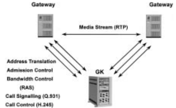
Fig. 10. Gatekeeper routed call signaling (Q.931/H.245).
