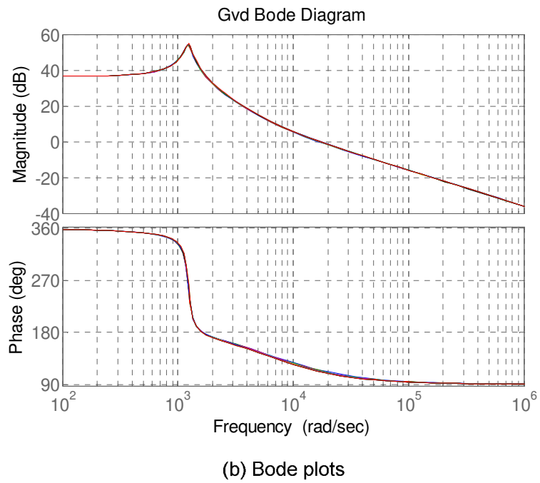
Figure A.5 Effect of load inductance variation on ZSC dynamics ( 200\mu H - 2000\mu H )
