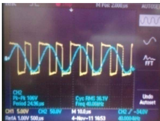
(b) PWM output for a 5 V, 40 KHz modulating signal
