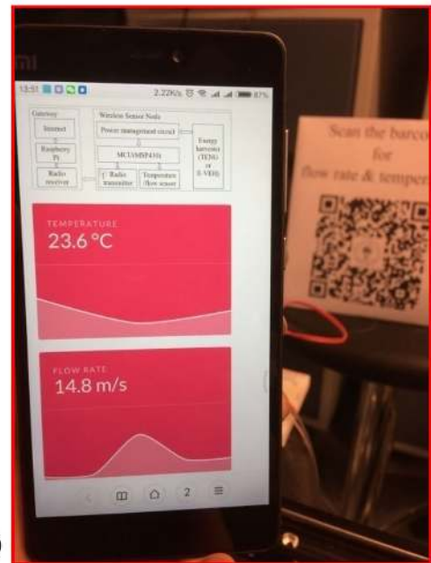
FIGURE 10. (a) A wireless sensing test for both the temperature and air flow rate in environment monitoring for 2.6 hours. The self-powered sensor node can acquire the sensing signals once per 140 seconds at an air flow of 14.7 \text{ m} \cdot \text{s}^{-1} ; (b) application in mobile phone.
