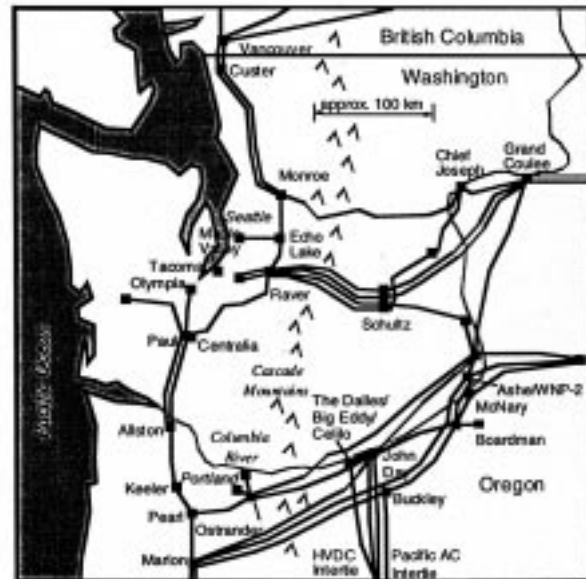
Fig. 1. Pacific Northwest 500-kV transmission network.
