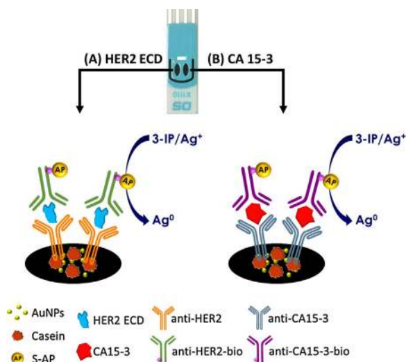
Fig. 1. Schematic representation of the immunoassay for (A) HER2-ECD and (B) CA 15-3 on a bi-SPCE-AuNP.
