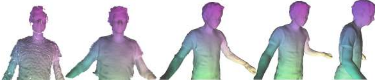
Fig. 8. Evaluation of tracking stability: surface points are colored according to the position in the canonical pose. Our non-rigid tracking maps each surface point close to its undeformed position. In case of tracking failures or drift, the surface would change its color over time (Color figure online)
