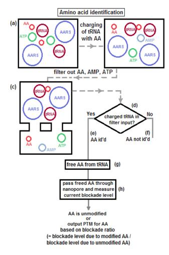
Figure 2. Schematic showing AA identification with tRNA followed by PTM identification with nanopore
