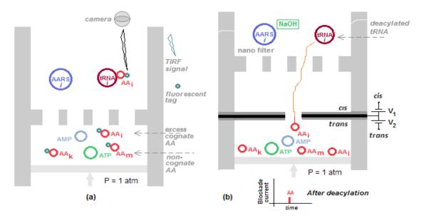
**Figure 3**. Detection of AA bound to cognate tRNA. (a) Optical detection of tag attached to AA with TIRF; (b) Electrical detection of AA after AA is freed from tRNA and passed through nanopore where occurrence of current blockade signals its presence.
