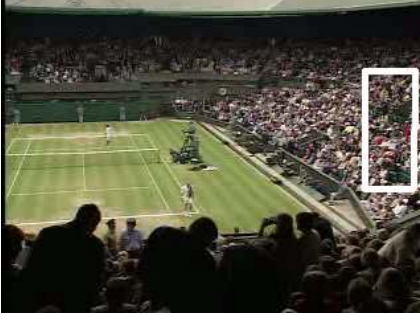
Figure 13. False positive in cluttered video regions. Because of the extreme over-segmentation of these regions, the tiny regions can be arbitrarily grouped to match any template.
