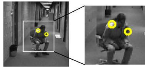
Figure 4. Space-time interest points are often found on highlights and shadows. These points are sensitive to lighting conditions and reduce recognition accuracy. This observation motivates our decision to apply volumetric features to the motion vectors rather than to the raw pixels.
