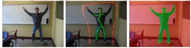
Figure 24. Illustration of how we generate model templates using an interactive video segmentation process similar to Wang et al. [65]. Given the training video (left), we draw a few strokes to label the foreground and background regions (middle), and graph-cut generates the complete segmentation mask (right).
