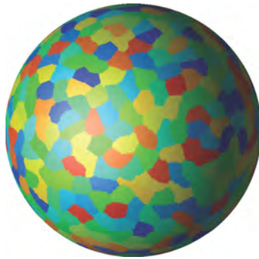
Fig. 11 Decomposition of a global SCVT mesh of 40962 generators into 642 blocks. The blocks can be distributed across computational nodes for implementation on high-performance architectures.
