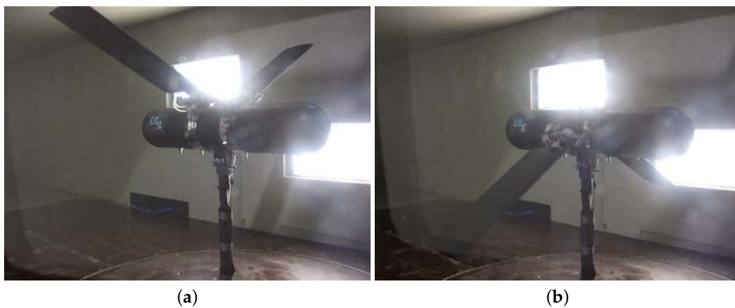
Figure 2. Maximum and minimum flap angles: (a) maximum flap; (b) minimum flap.
