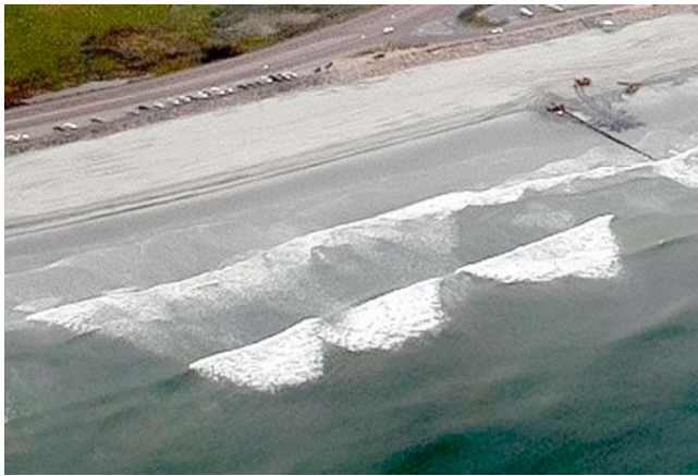
Figure 1. Photograph of breaking waves (propagating toward the shore from lower-right to upper-left) showing the triangular patches of residual white foam marking the location where breaking occurred. As the waves break, they transfer momentum to the water column and generate vorticity. The initially small breaking region on the lower right expands as the wave moves toward shore on the upper left. This pattern is typical in the surfzone, with the shape of the triangle varying with wave conditions.
