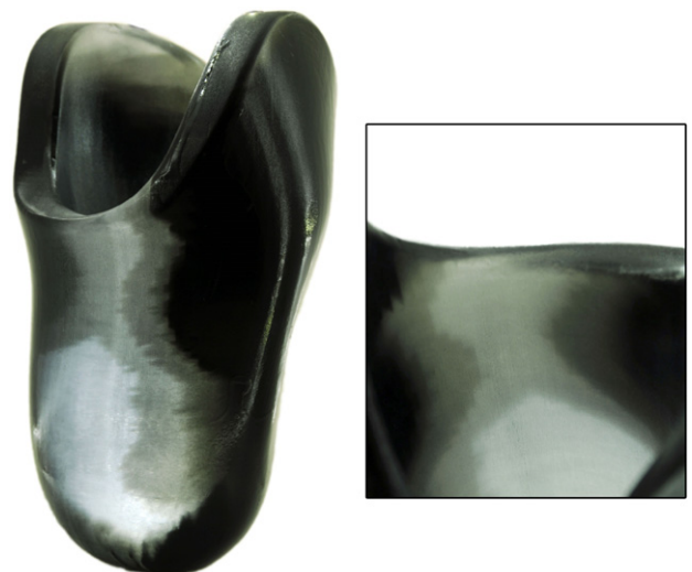
Fig. 8. Fabricated socket (maximum dimensions: 121 * 124 * 223 mm) and detail view illustrating the achieved material transition.
