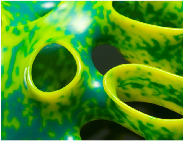
Fig. 2. Portion of a multi-material printed object from the exhibition “Imaginary Beings: Mythologies of the Not Yet”. Produced by StratasyS using an Objet500 Connex printer.
