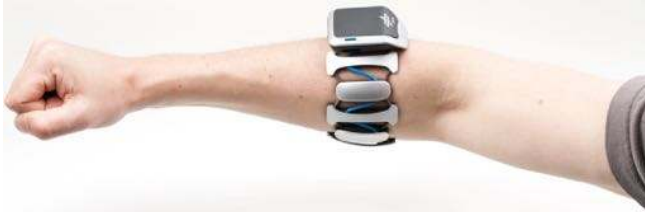
Figure 14. The VibroTac provides tactile feedback on the arm using six vibration motors equally distributed. The variation of the rotation frequency of the motors enables a higher resolution than the six segments.
