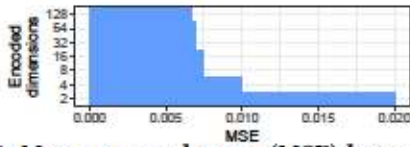
Figure 11: Mean squared error (MSE) between validation dataset and reconstructed sequences after encoding for a variable number of latent dimensions.
