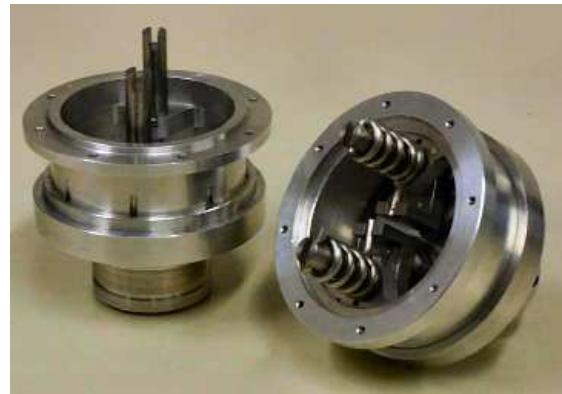
Fig. 9. VSA-II prototype, open up. The prototype integrates the non-linear elements needed to obtain the variable stiffness. It is composed of two equal halves, each half contains two 4-bar mechanism to allow internal stress to be distributed more evenly along the structure.
