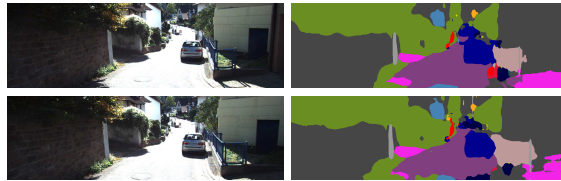
Fig. 5. Consecutive frames from KITTI sequence 10 with inconsistent semantic segmentations. Increasing the uncertainty \sigma in the semantic segmentation places less weight on our semantic constraints and allows us to handle such scenes. In general, small values for \sigma are preferable if shape details are consistent.
