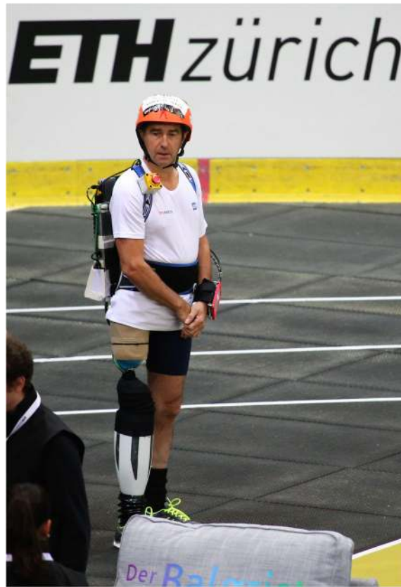
Fig. 5 The VUB-CYBERLEGS pilot. Our pilot, Michel de Groote wearing a complete VUB-CYBERLEGS Beta Prosthesis system during the CYBATHLON. The system consists of the prosthesis, a backpack with the computer and battery, and an arm mounted touchscreen control
