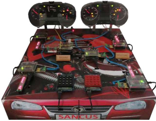
Figure 6: Hardware-in-the-loop application scenario with original instrument clusters and Sancus-enabled ECUs.
