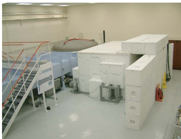
Figure 15. The Petawatt target area complete with radiation shielding.
