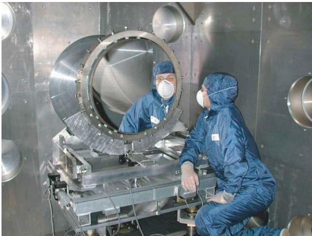
Figure 9. The F#3.1 off-axis parabola installed in the Petawatt target interaction chamber.
