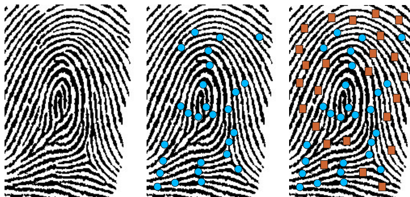
Figure 5: Schematic diagram of the biometric encryption scheme of Clancy et al. (2003). Left a raw fingerprint image is enrolled. Middle minutiae points (circles) are used to encode the value of a polynomial representing the secret. Right chaff points (squares), sufficiently far from minutiae, are used to encode random values of the polynomial.
