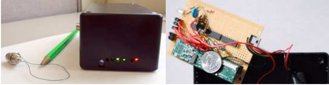
Fig. 1. Our assembled PICCAL credit card emulator
