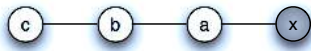
Figure 5. Limitation of link spoofing: malicious router X can not obtain the identity of router c directly through NHDP.
